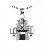
This sealed system snubber is indicated where extremely accurate response is required; or where it is desirable to disassemble the diaphragm seal for cleaning purposes. This ability is particularly important where it is being used on materials highly contaminated with solids inclusions which might tend to pack under the diaphragm.
